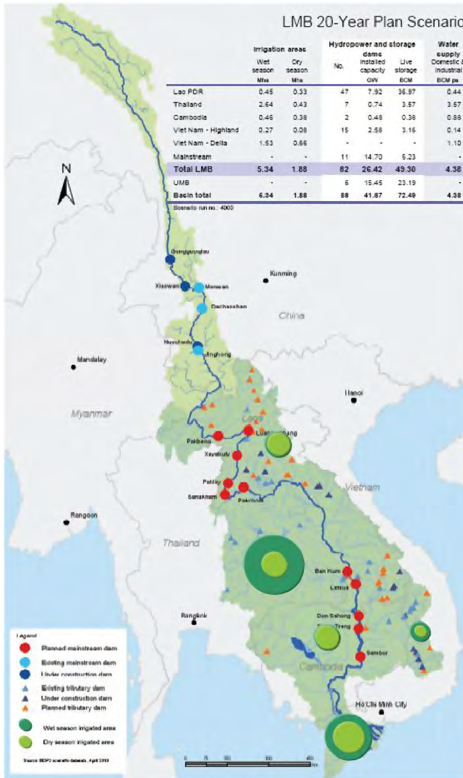
Fig. 1. Location of the 30 planned tributary dam plus 11 planned mainstream dams (from Mekong River Commission, 2011).
